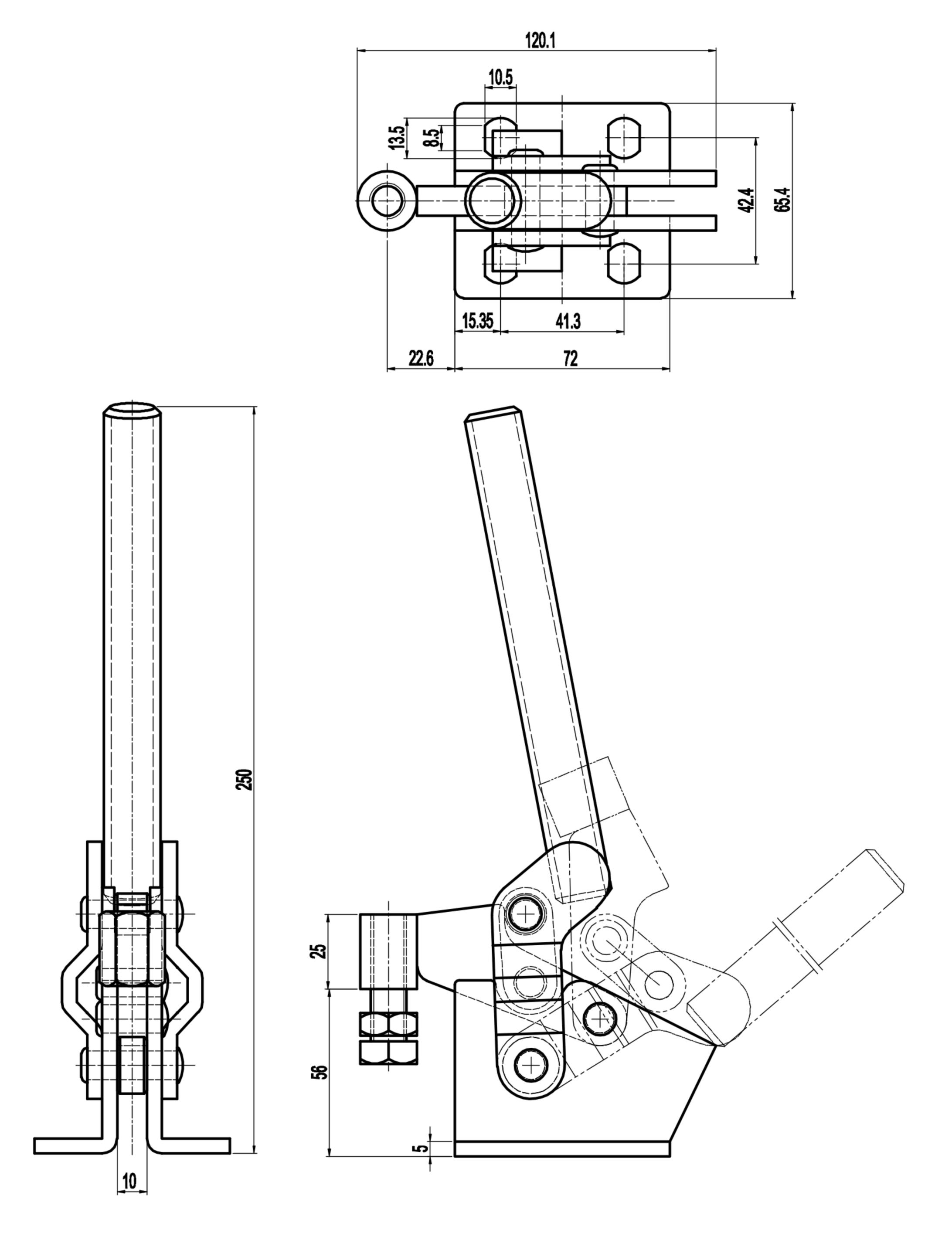
BAR OPENS:67.5° HANDLE OPENS:60° SPINDLE SUPPLIED:CH—SA—125017
